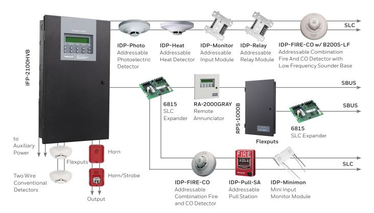
Flexput Circuits - Flexible input or output circuit that you can conveniently program to be used for Notification Appliance Circuits, Auxiliary Power, or as a conventional input circuit. With auxiliary power, it can be selected as constant power, door power, or resettable smoke power. The Flexput circuits provide the utmost versatility without the added expense of additional modules, a perfect fit for retrofitting an existing conventional system when budgets are a concern.
